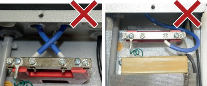
Do not allow the high voltage cable to form a loop or crisscross in the power unit. The cable must go straight into the terminal screw.
