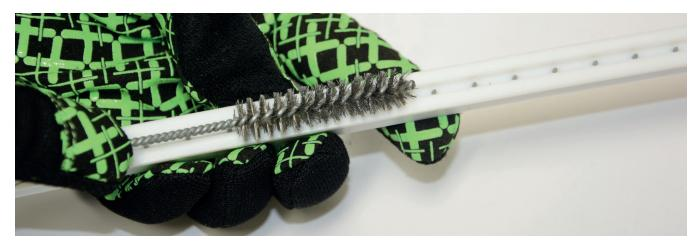
12. Using a moderately stiff brush or compressed air, clean the emitter points on the face of the bar to remove any metal fragments, filings or debris.
