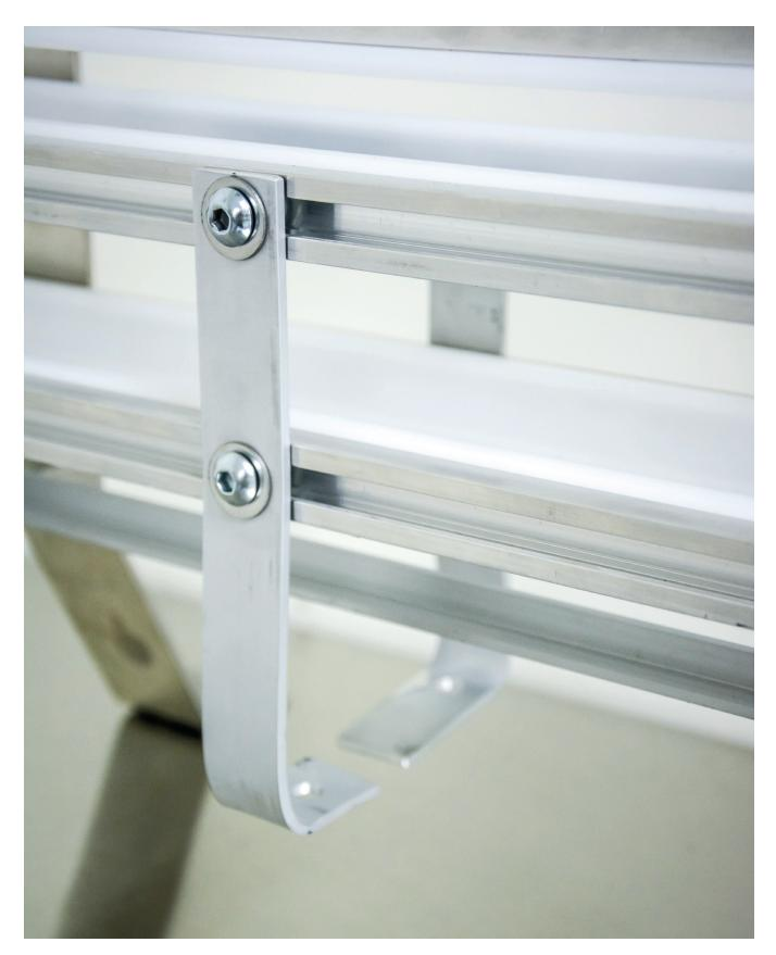
2. Attach one right and one left bracket to conveyor rails, directly across from each other.
