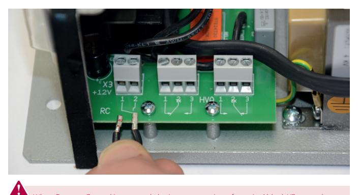
When Remote Control is not used, the interconnection of terminal block X3 must always be in place.
