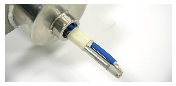
15. Remove the tape and pull dowel or metal rod from air delivery device. Pull remaining blue wire through the small opening, until the ionizing bar and metal housing are fully inserted and the metal housing butts against the end cap of the air delivery device. Align the emitter points of the ionizing bar in the direction of the air discharge; and align the nut-serts on the metal housing with the screw holes on the air delivery device (180° from the air discharge).
