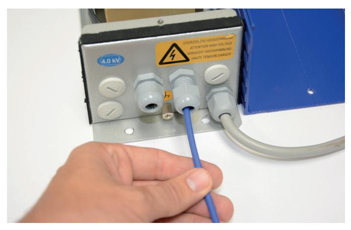
10. Push the blue high voltage cable from the air delivery device into the power supply, through the gland nut.
