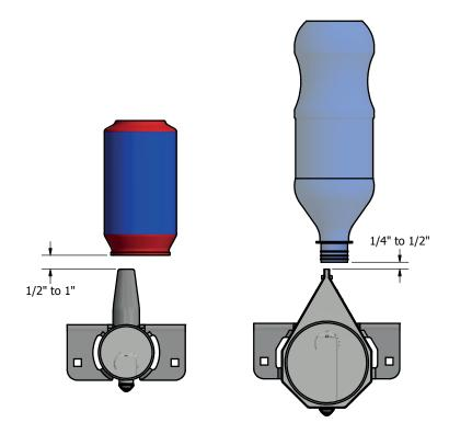
6. Adjust knife or nozzle to bottle or can opening as shown above, by shifting on mounting bracket.
