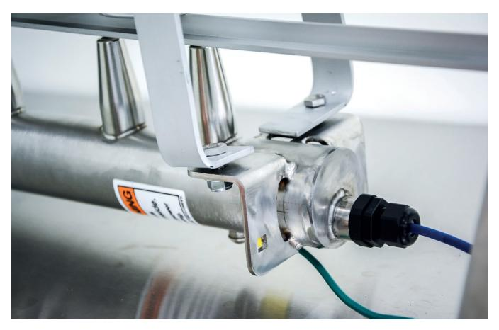
4. Attach knife or manifold to brackets.
