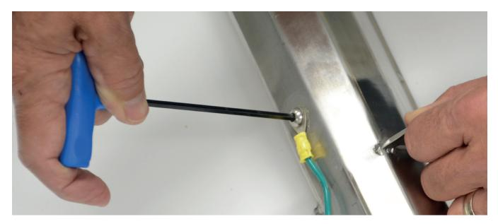
16. Using the ¼" x ½" screws, replace the ground wire while simultaneously securing the power bar inside the device. Loosely tighten the screw.
