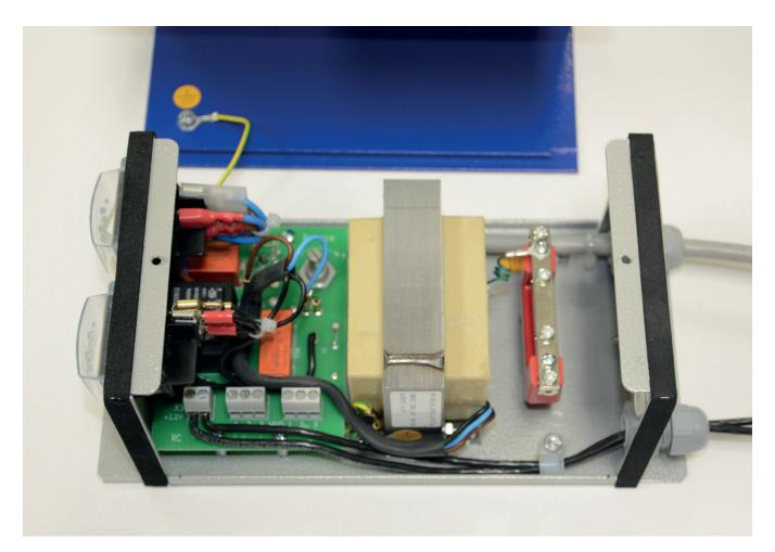
b. Feed the wiring through the gland and lay it as far as possible from the high voltage terminal block, and connect the wiring to terminal block X3.
